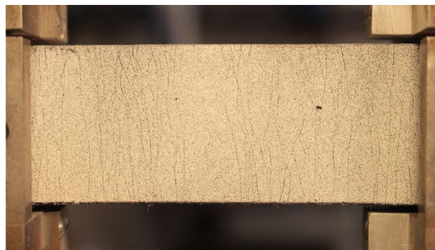
Fig. 1 Example of a multiple crack structure
