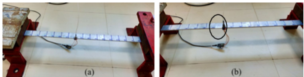
Fig. 3 Experimental setup of the fixed beam using MPU6050 and the conventional accelerometer: (a) healthy beam; (b) beam with a subtracted mass shown inside circle
