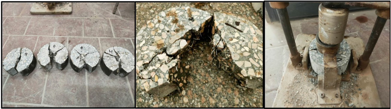
Fig. 16 The shapes of failure on hybrid polypropylene reinforced concrete under impact load
