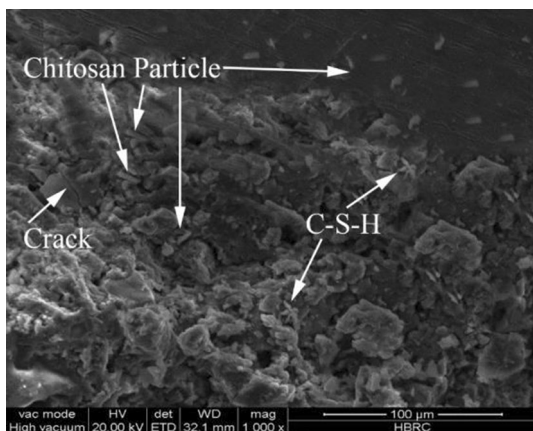
Fig. 14 SEM images of chitosan-based concrete
