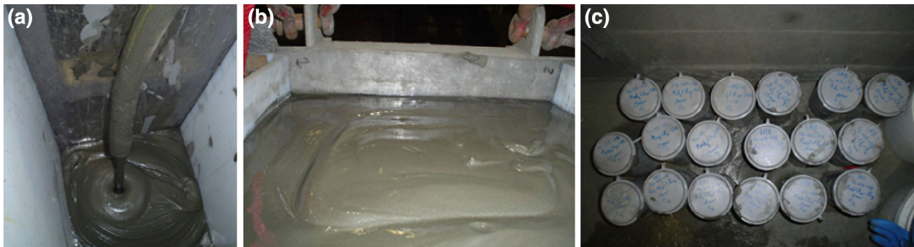
Fig. 7 Photographs showing the columns filling and plastic molds filled with CT1 and CT2 paste backfill
