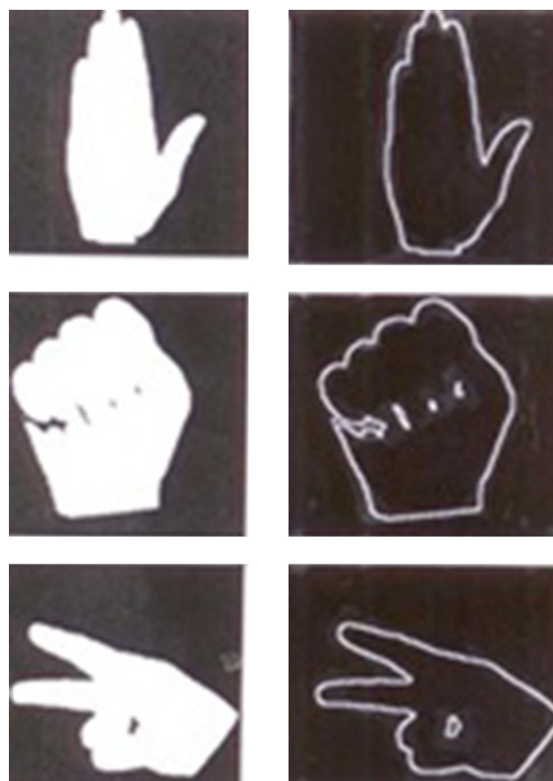
Fig. 6 Sobel edge detection for Open, Close and Cut
