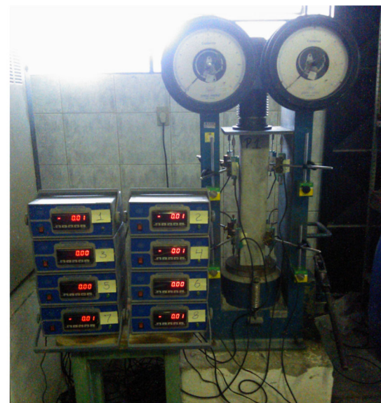
Fig. 8 Column P1 positioned in the press before the test
