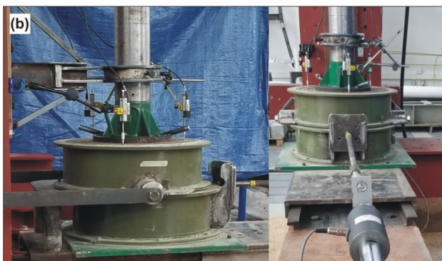
Fig. 3 Large direct shear device: a schematic diagram and b photos of the large direct shear box
