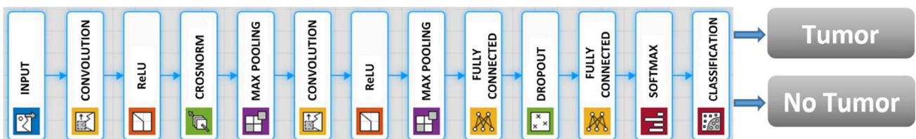
Fig. 2 Architecture of the proposed CNN model for Classification-1 task
