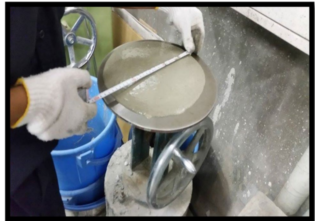
Fig. 3 Mortar flow photo
