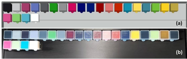
Fig. 1 First batch samples on print bed. a In GrabCAD print workspace. b Printed samples in J750 print bed (colours not to scale)
