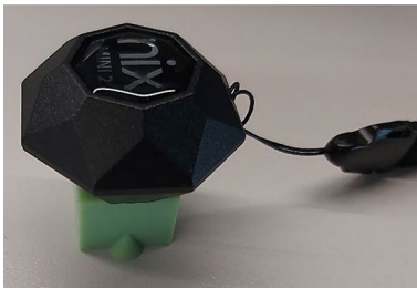
Fig. 3 Sample scanning with Nix mini 2 colour scanner
