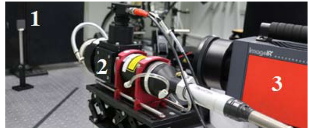
Fig. 4 Thermographic set-up: specimen (1), excitation source widened laser beam, optic for 39 \times 39 \text{ mm}^2 (2), Thermal Imaging Camera Infratec ImageIR 8300 hp (3)
