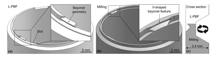
Fig. 7 Bayonet design with a L-PBF geometry (male), b milling geometry (female), c schematic assembly design
