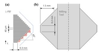
Fig. 5 Geometric constraints for a L-PBF with a layer thickness of 40  $\mu$ m, allowable overhang of 45°, min. wall thickness of 0.3 mm; b milling tool with a groove width of 0.2 mm, chamfer of 45°, max. depth of 1.5 mm; dimensions not to scale; expected L-PBF roughness in dashed red, ideal milling contour in dotted blue
