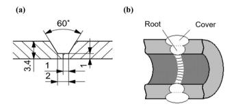
Fig. 4 a Standard weld preparation geometry, b root and cover pass
