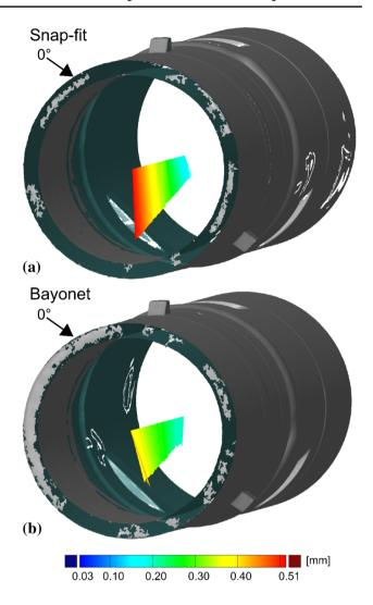
Fig. 12 3D scan results after welding of  $\bf a$  snap-fit design and  $\bf b$  bayonet design with measured center lines of the L-PBF cylinders in relation to the target center lines. A scaling factor of 30 for the shown deviations was used to improve visibility.  $0^{\circ}$  indicates the start position of the root weld
