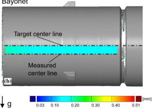
**Fig. 11** 3D scan results before welding of **a** snap-fit and **b** bayonet design with measured center lines of the L-PBF cylinders in relation to the target center lines. A scaling factor of 30 was applied to improve visibility
