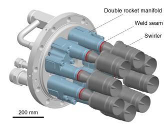
Fig. 1 SGT-8000(H) combustion system with weld seams between swirlers and manifolds highlighted in red
