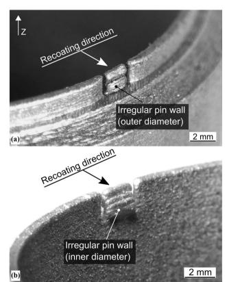
Fig. 9 Deformed snap-fit pins a on the outer diameter, b on the inner diameter, with recoating direction
