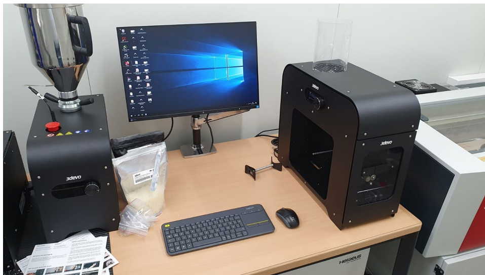
Fig. 2 Desktop Recycling setup “SHR3D IT” shredder, “AIRID” polymer dryer and “PRECISION” extruder. Desktop recycling plant with shredder, dryer and extrusion line for the production of filament from various polymers in small-scale industry and research
