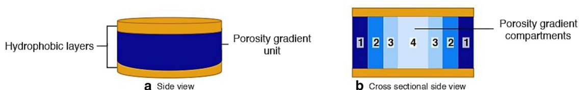
Fig. 5 Schematic representation of a material gradients tablet. A different porosity degree allows a faster erosion when the surface area decreases resulting in a constant drug release Picture adapted from [20]
