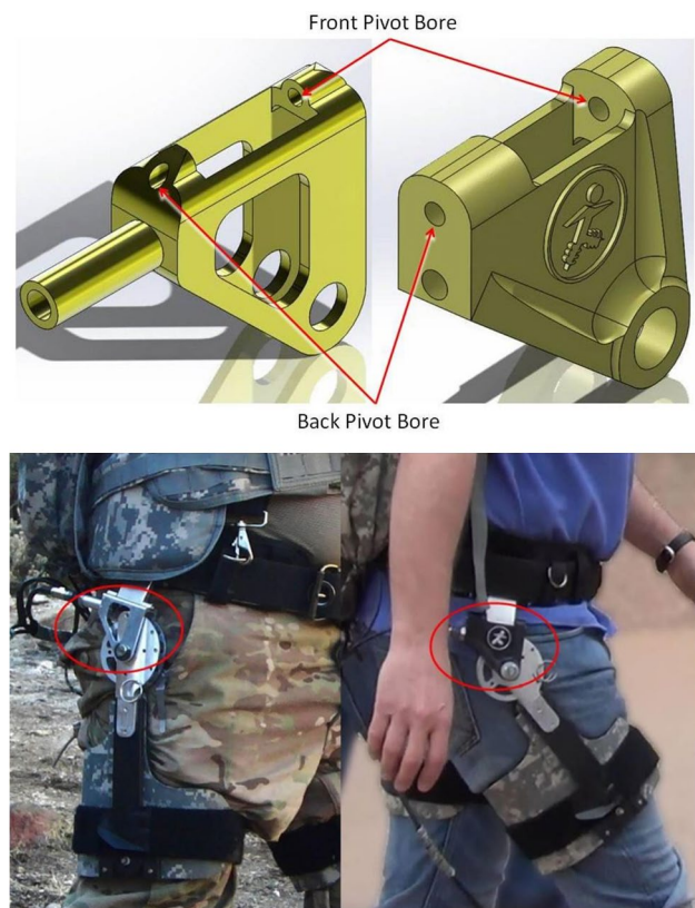
Fig. 8 The CNC-machined part (left), the 3D-printed part (right) [41]
