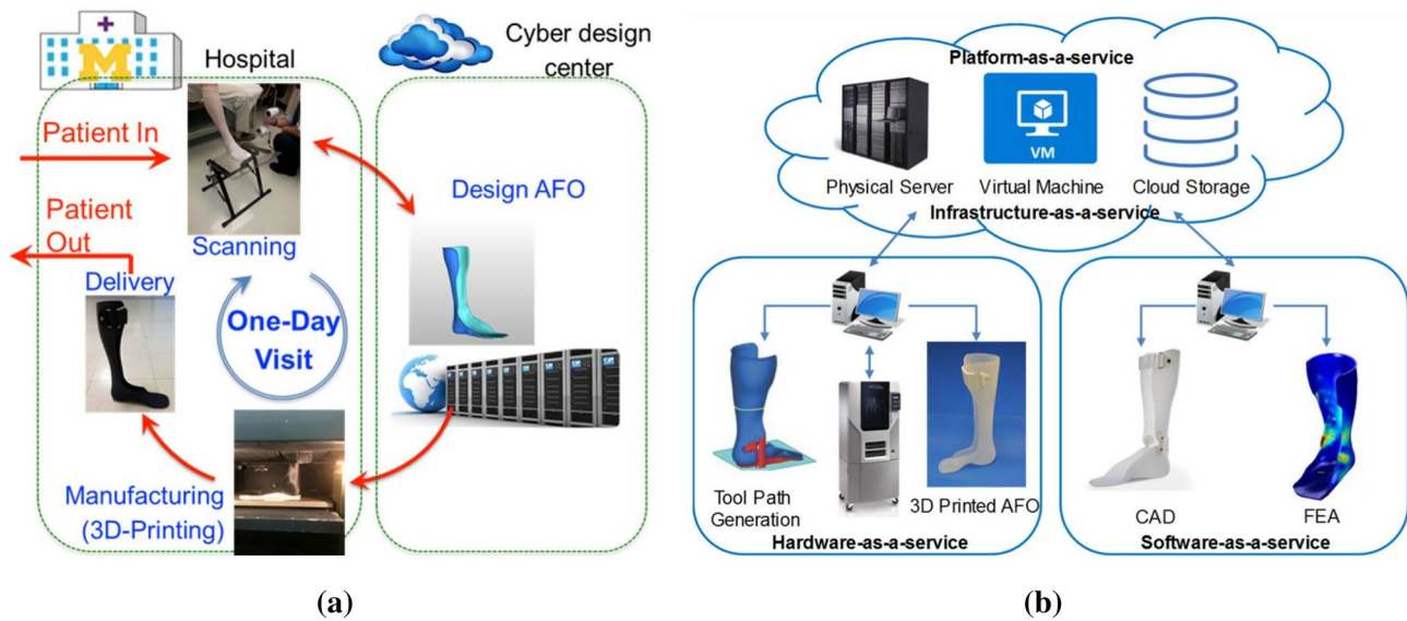
Fig. 3 a Overview of the CDAM system for custom AFOs. b Illustration of the interaction between the hardware and software systems with the cloud storage system [24]
