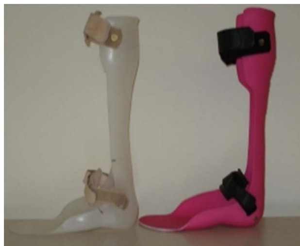
Fig. 11 The PP ankle–foot orthosis (left) and the additive manufactured ankle–foot orthosis (right) [51]
