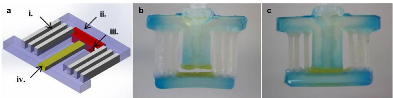
Fig. 4 A smart valve is created by 4D printing [3]
