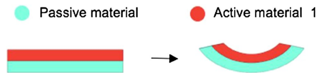
Fig. 15 Conventional multi-material printing to create a bilayer of an active and a passive layer
