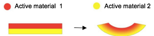
Fig. 16 Functionally graded AM heterogeneous composition of two active materials
