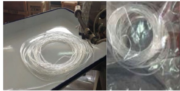
Fig. 3 Extruded TPU filament through single-screw extrusion
