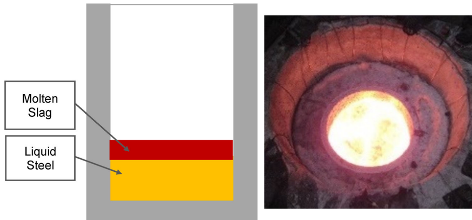
Figure 20. Left: a cross section of crucible in induction furnace and right: image of foamy slag during melting experiment.
