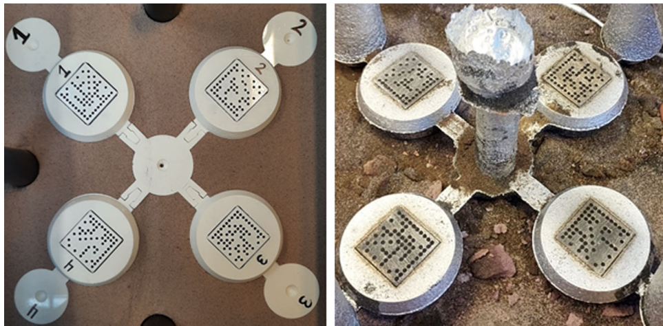
Figure 14. Sand mold configuration of the parts with different unique datamatrix id codes (left) and after shakeout (right).
