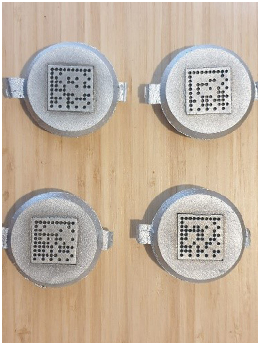
Figure 11. Multiple unique tags on the same part.
