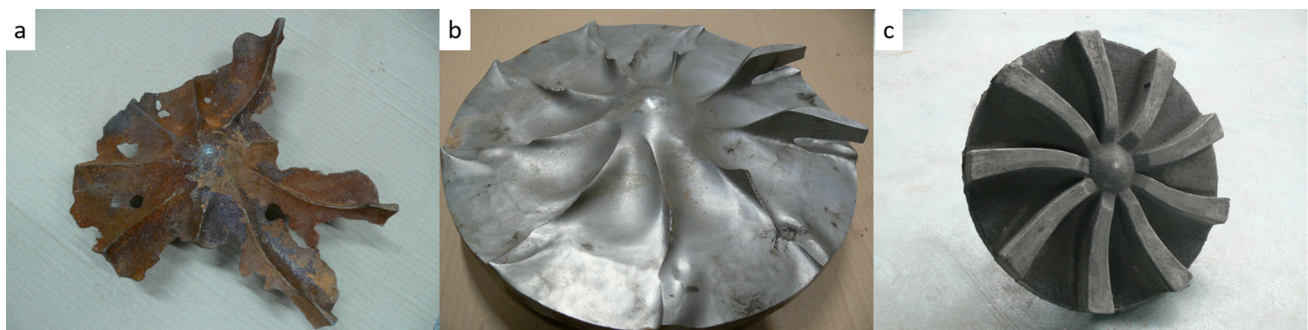
Figure 1. Pump impeller with visible traces of abrasive wear and pitting corrosion after a period of operation in an environment rich in chlorides—chromium cast iron (a), pump impeller after the period of operation with visible traces of abrasive wear after the period of operation in the absence of corrosive factors—chromium cast iron (b), and pump impeller after casting in the raw state—silicon cast iron (c).
