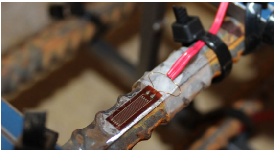
Fig. 2 Strain gauge attached to a reinforcing bar
