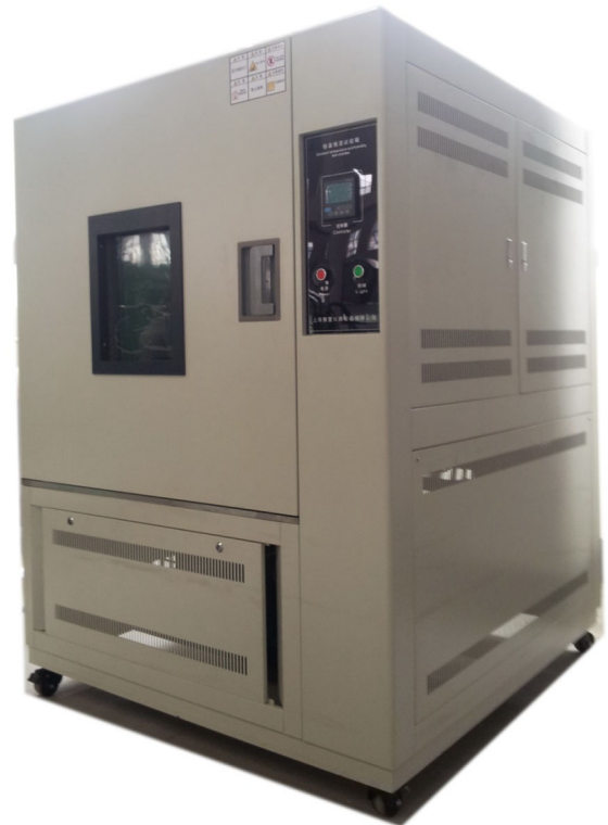
Fig. 3 Specimen curing device
