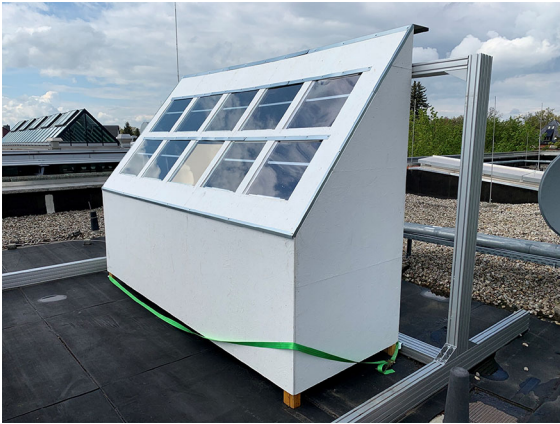
Fig. 13 Test rig with specimens on a flat roof
