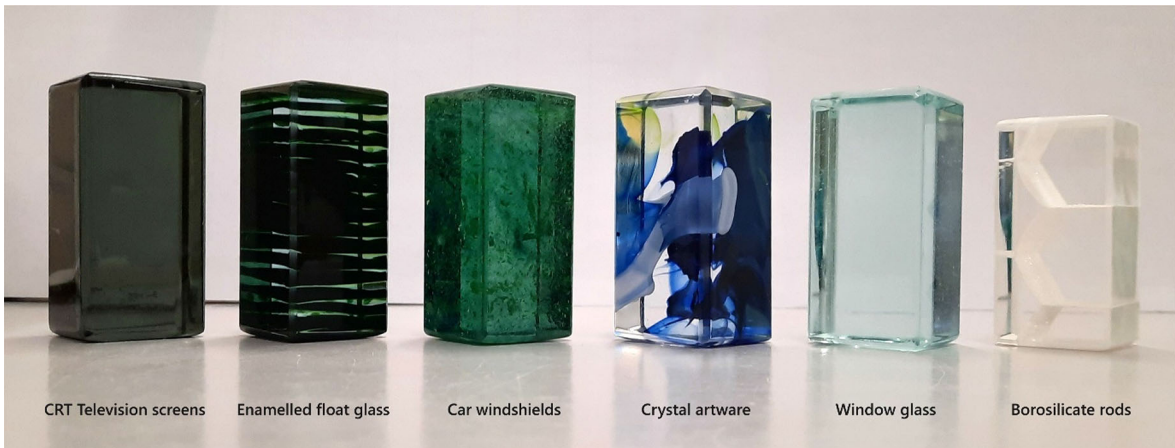
Fig. 29 Wide range of kiln-cast glasses evolved from the recycling of various different glass waste streams. Systematic validation is required to identify the mechanical properties and quality grade of each recycled cast glass and provide the industry with design data
