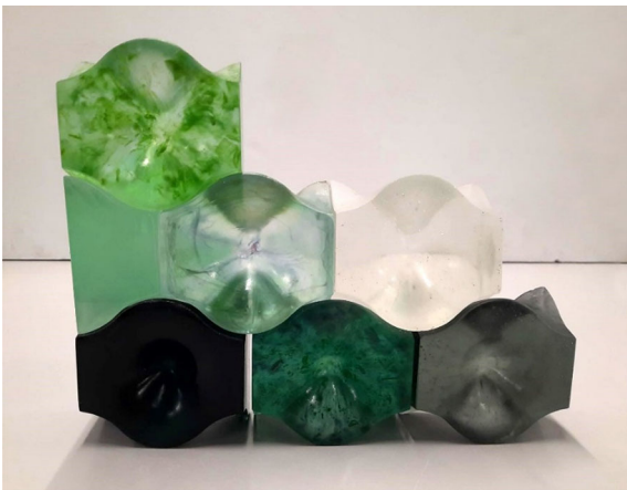
Fig. 30 Structural cast glass components out of different glass waste streams, to be used in an interlocking wall system
