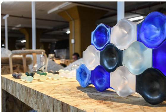
Fig. 17 prototype of interlocking cast glass units, as described in (Oikonomopoulou et al. 2018) that can evade the use of adhesives
