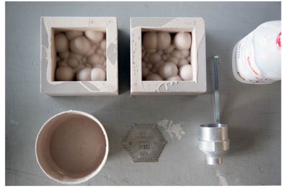
Fig. 2 Immersion coating process with Zirkofluid® coating
