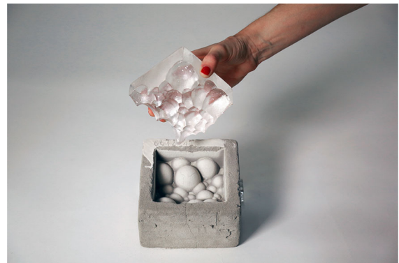
Fig. 4 Kiln cast glass part (10 × 10 × 8 cm) removed from 3D-printed mold after annealing
