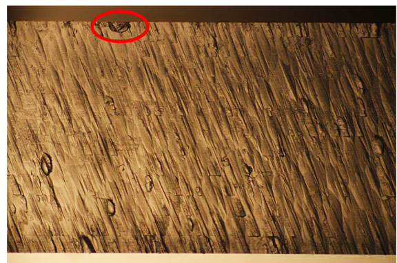
Fig. 12 Machined surface of a PMMA tensile specimen 25\times magnified, showing certain defects from manufacturing
