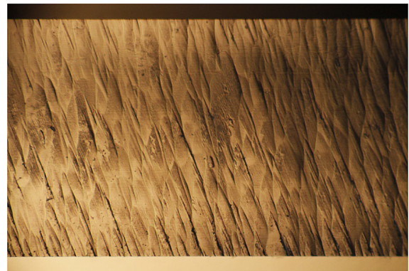
Fig. 11 Machined surface of a PMMA tensile specimen 25\times magnified, resulting from a sufficient milling process. Height is the 3 mm thickness of the extruded plates
