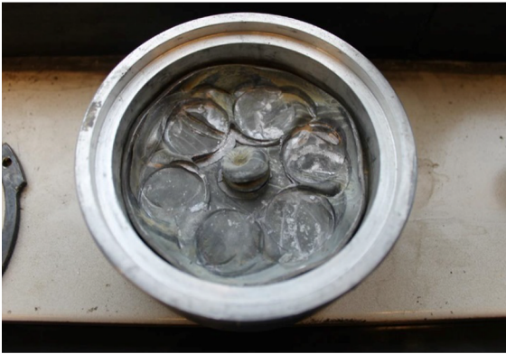
Fig. 8 Load introduction pre-study: lead interlayer in an end cap, photographed after loading and disassembling adhesively bonded glass bundle
