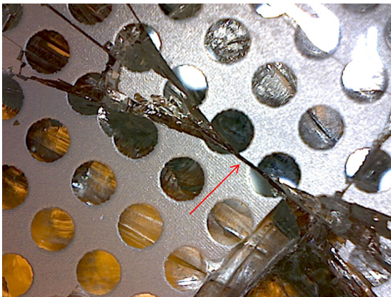
Fig. 13 Fracture origin for Specimen 5 from Sample 4
