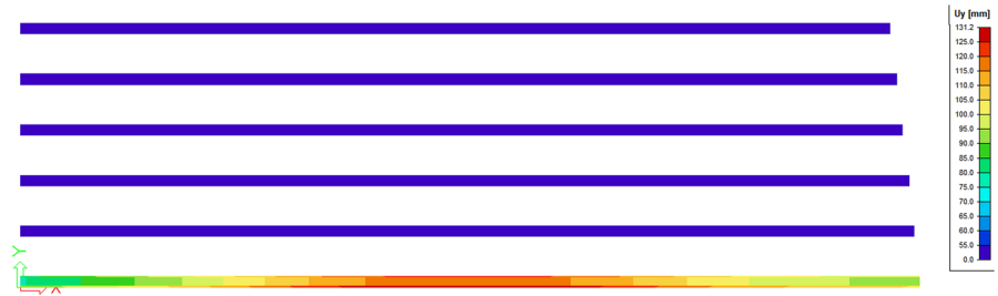
Fig. 11 Theoretical situation without glass: lateral deformations due to wind loads over 130 mm in the front beam
