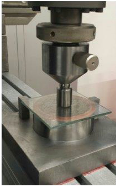
Fig. 10 Photo of bending test set up
