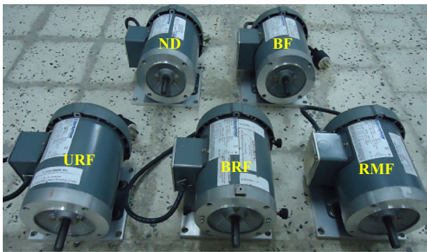
Fig. 5 Five Induction motors with individual faulty conditions (ND no defect, BF: bearing fault, URF unbalance rotor fault, BRF bowed rotor fault and RMF rotor misalignment fault)
