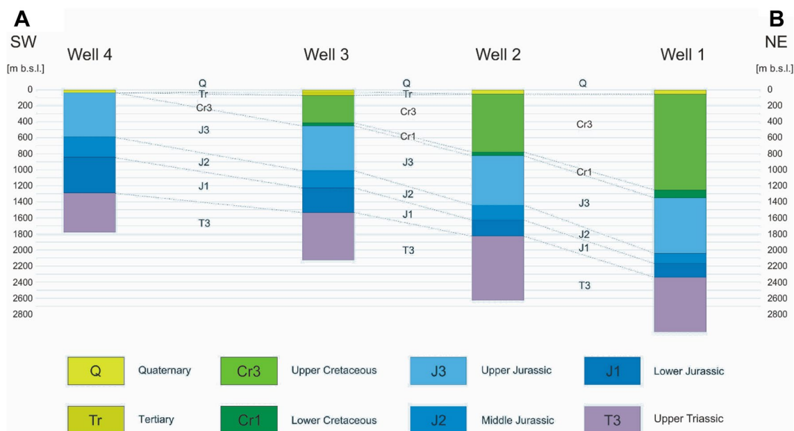
Fig. 3 Stratigraphy and thickness of mesozoic, tertiary, and quaternary strata along the A–B cross section in Fig. 2
