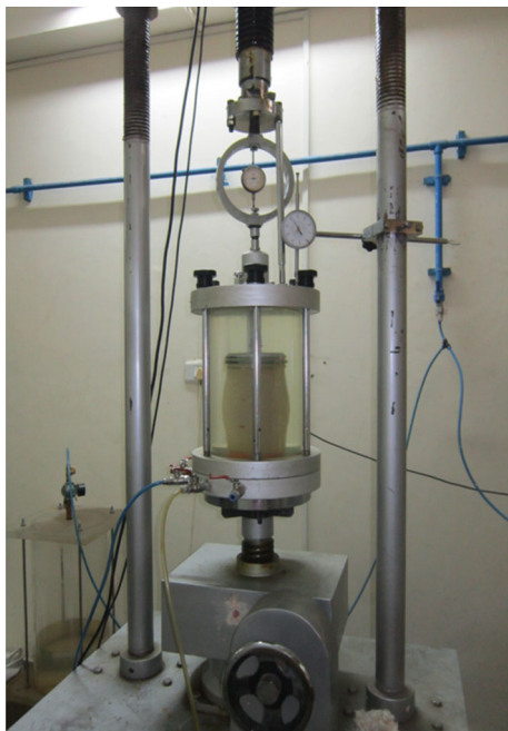
Fig. 3 Triaxial testing with loading frame and large scale triaxial cell
