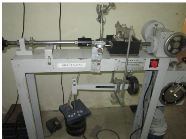
Fig. 4 The direct shear pull out test setup
