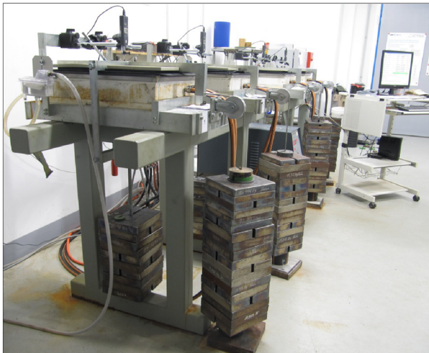
Fig. 3 Shear creep rupture test devices
