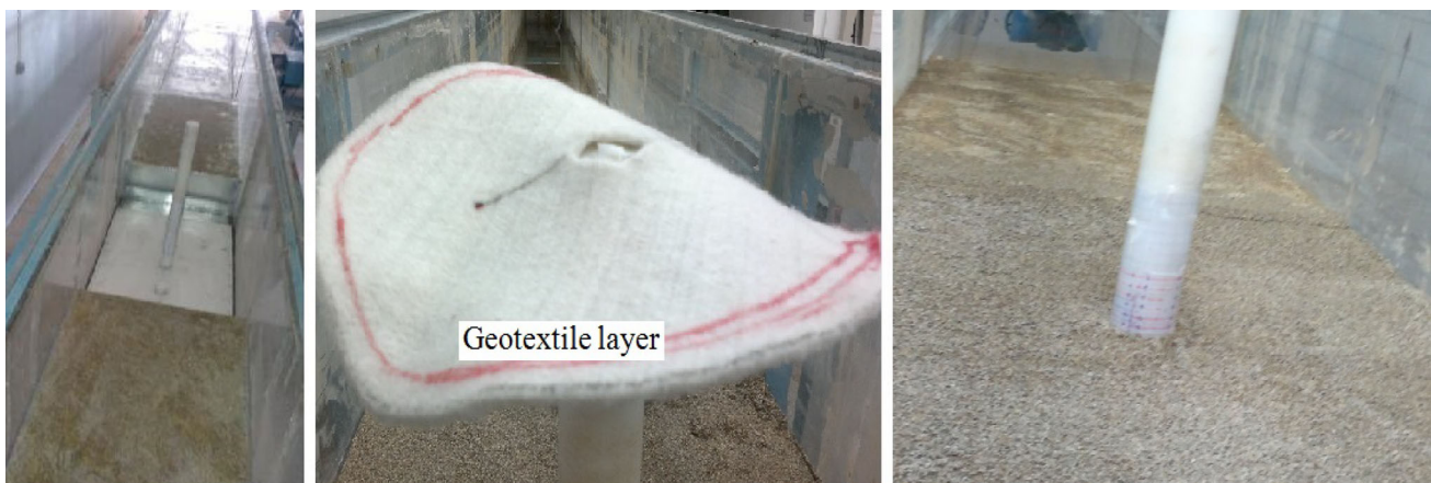
Fig. 1 Pier model installation in the flume
