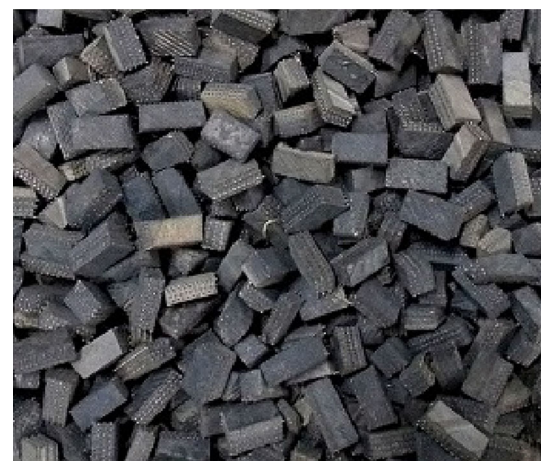
Fig. 4 Typical tire chips used in this study
