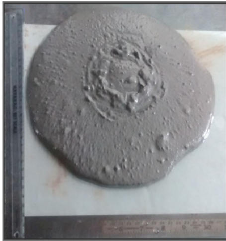
Fig. 4 Flowable mix for measuring spread diameter
