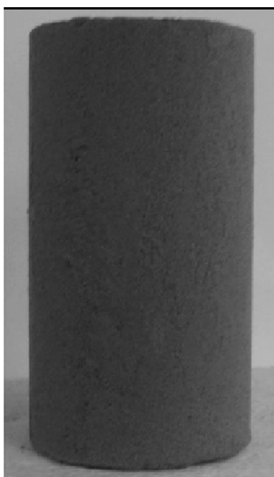
Fig. 6 Ejected sample from mould
