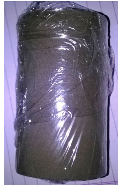
Fig. 7 Sample wrapped with cling film
