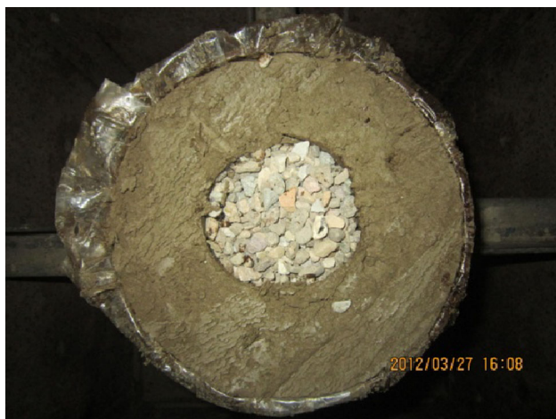
Fig. 2 Unit cell with stone column
