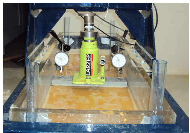
Fig. 7 Model footing load test arrangement under submerged condition
