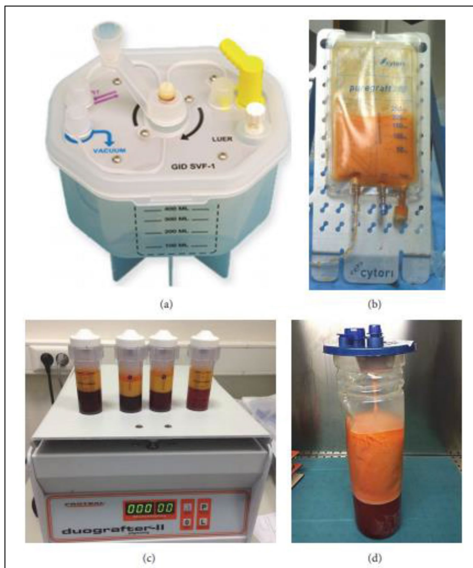
Fig. 2 Devices used for SVF and SVF-MAT isolation. a GID-SVF1. b Puregraft 250. c Stem.pras. d Reference method. Adapted from Jonathan Rodriguez et al., 2017 [35]
