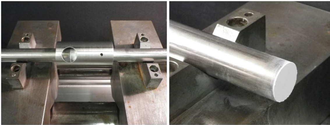
Fig. 3 Left: photograph of revealed HMX explosive layer sitting between the input-bar and the output-bar. The explosive layer (white) is seen through the filling port of confining sleeve. Note the smaller port to the right of the sleeve, normally used to house an optical fibre for reaction sentencing and temperature measurement. Dur-
