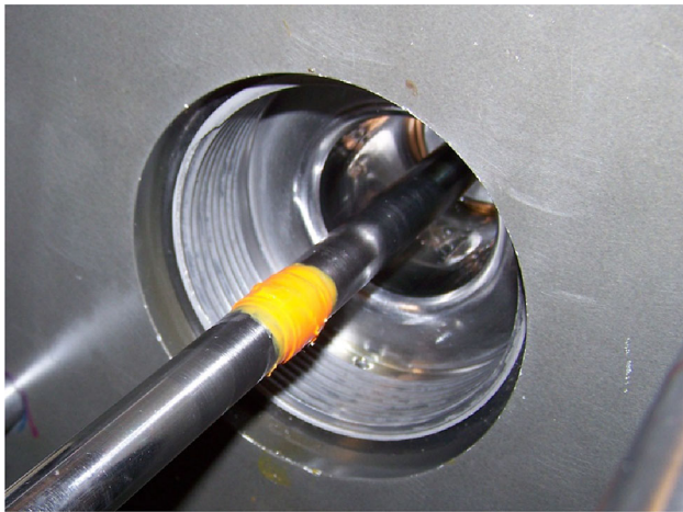
Fig. 3 A sealed acrylic specimen ready for an experiment
