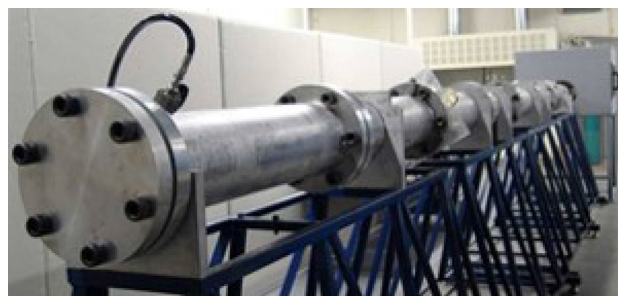
Fig. 2 Shock tube facility
