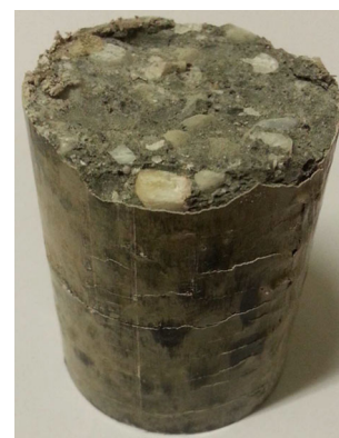
Fig. 9 Image of a wet high-strength concrete specimen tested in dynamic quasi-oedometric compression
