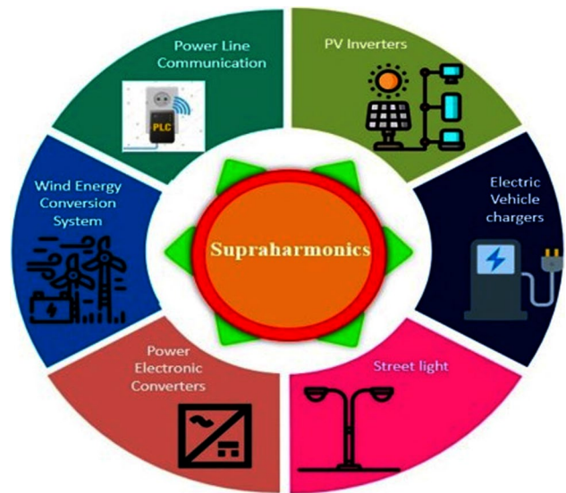
Fig. 7 Sources of Supraharmonics
