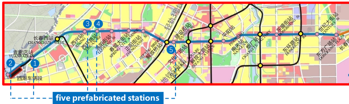
Fig. 8 Five prefabricated stations on Changchun Metro line 2
