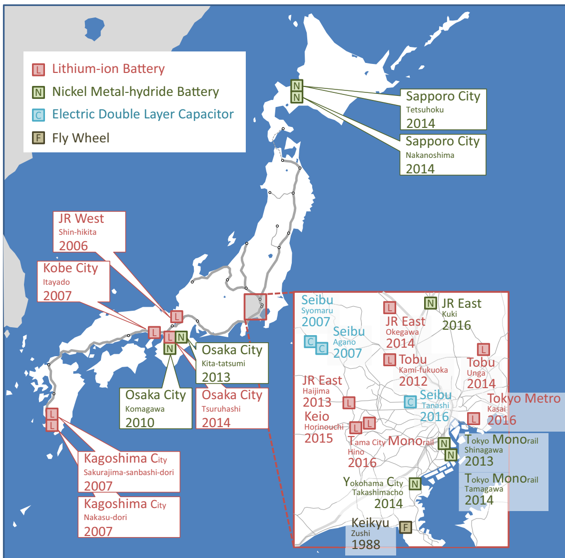
Fig. 8 Existing energy storage systems in DC traction power supply system in Japan
